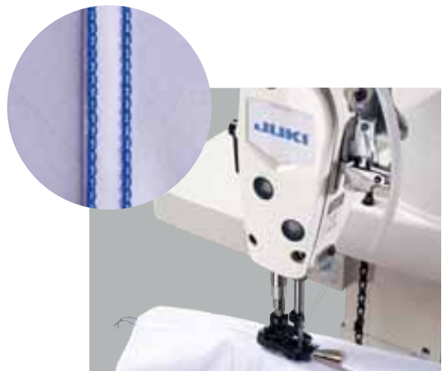
● Low-tension sewing ensures balloon stitches with a soft feeling.
